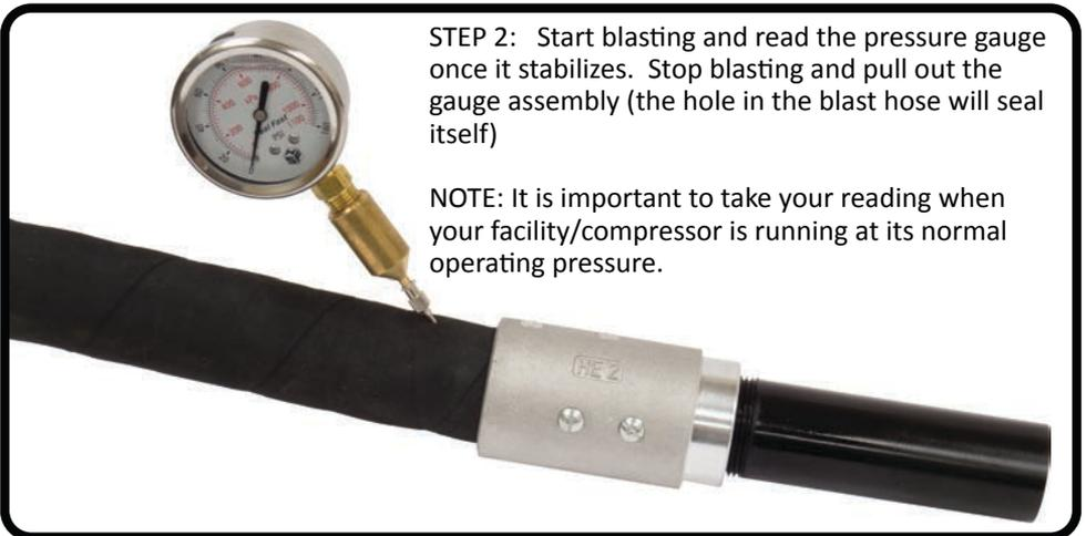
**STEP 2:** Start blasting and read the pressure gauge once it stabilizes. Stop blasting and pull out the gauge assembly (the hole in the blast hose will seal itself)
