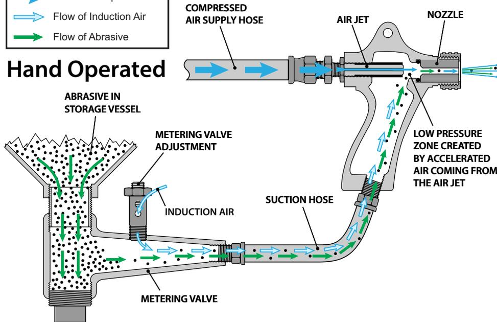
Suction blast systems work by drawing abrasive to the nozzle using suction instead of pushing it through a blast hose with compressed air.
