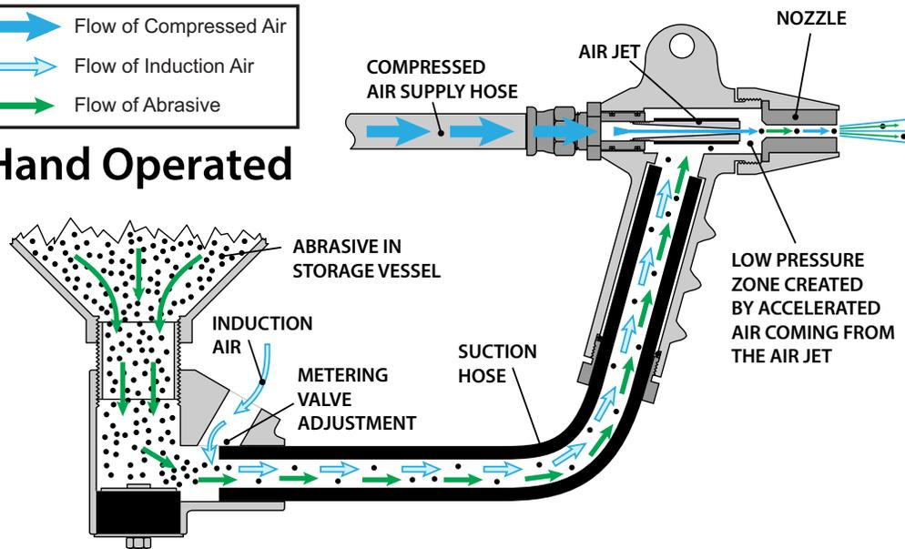
Suction blast systems work by drawing abrasive to the nozzle using suction instead of pushing it through a blast hose with compressed air.
